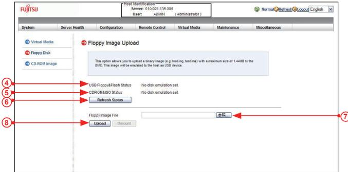
4. *USB Floppy & Flash Status* displays the status of a USB floppy or a flash device.
